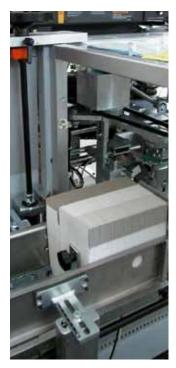
The **AV30** is a top-load, intermittent motion cartoning machine suitable for manual or automatic packaging of pharmaceutical, nutraceutical, cosmetic and food products into pre-glued cartons.
