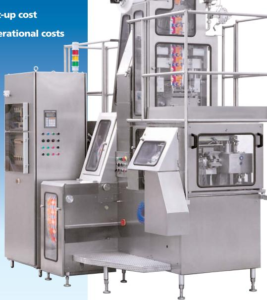
The SA-50/2 Aseptic filler forms, fills and seals packages in one continuous operation in sterile environment.
